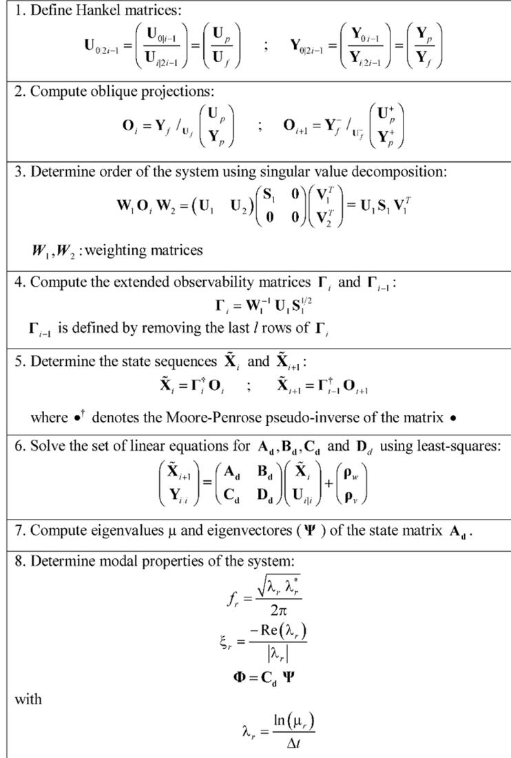
Figure 3. Schematic overview of the DSI system identification method (adapted from [12]).
