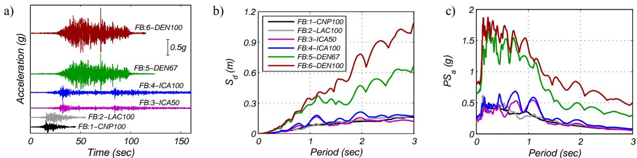
Figure 2. Input ground motions achieved on the shake table: (a) Acceleration time-histories; (b) Elastic displacement response spectra ( $\xi=5\%$ ); (c) Acceleration response spectra ( $\xi=5\%$ ).
