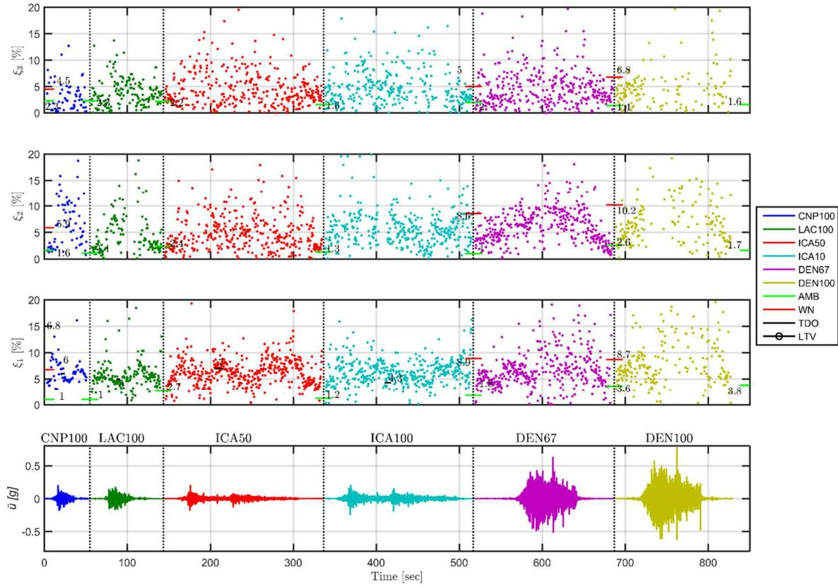
Figure 6. Temporal evolution of the damping ratios identified for first three longitudinal modes.
